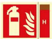
FE.013 Halon fire extinguisher
