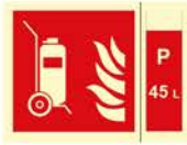
FE.037 Powder wheeled fire extinguisher
