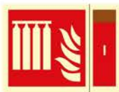
FE.050 Extinguishing battery inergen
