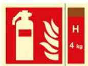
FE.014 Halon 4 kg fire extinguisher
