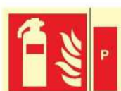
FE.016 Powder fire extinguisher
