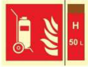
FE.035 Halon wheeled fire extinguisher
